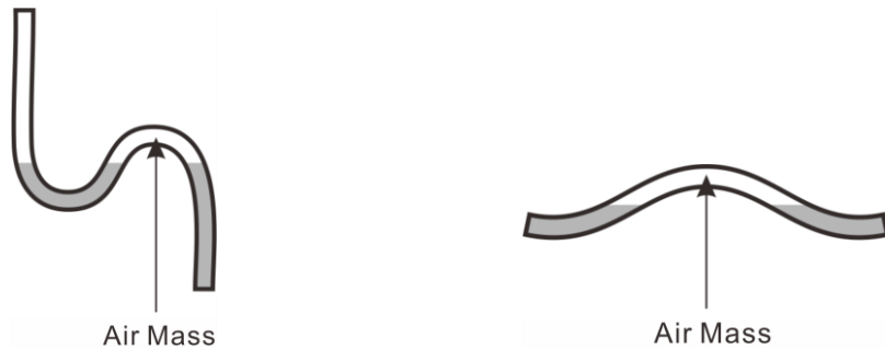
Fig.6 – Incorrect Pipe Connection
